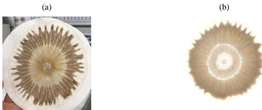
Figure 1: Untreated soil chromatogram (a). Soil chromatogram with SAF application (b).
